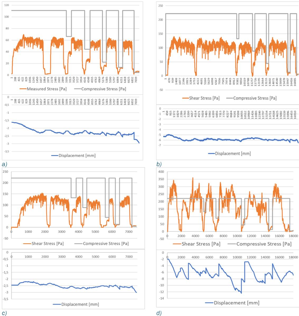
Figure 15. Raw data time series obtained with the Schulze Ring shear tester, 5kg pre-shear load: a) 6 mm wooden spheres, standard lid; b) 10 mm wooden spheres, standard lid; c) 10 mm wooden spheres, modified lid; d) Iron ore pellets, modified lid.
