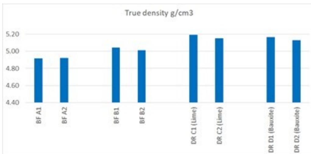
Figure 5. True or absolute density measurement of BF and DR grade pellets.
