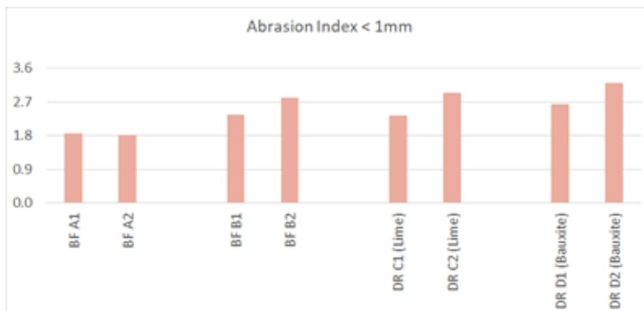
Figure 8. Abrasion index of BF and DR grade pellets.
