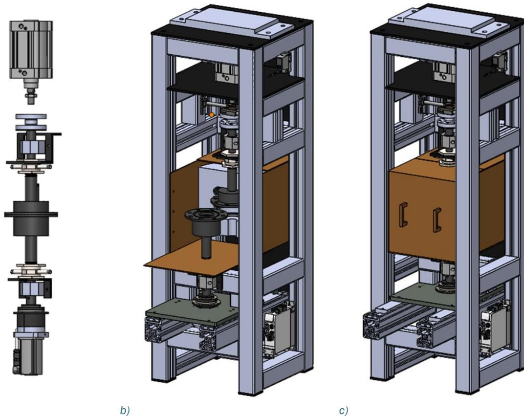
a) Figure 19. The sequence of elements needed to conduct tests; b) the opened device for cell loading; c) the device in operation.
