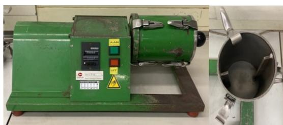
Figure 6. Small drum mini- ASTM device for measuring tumbler and abrasion index.
