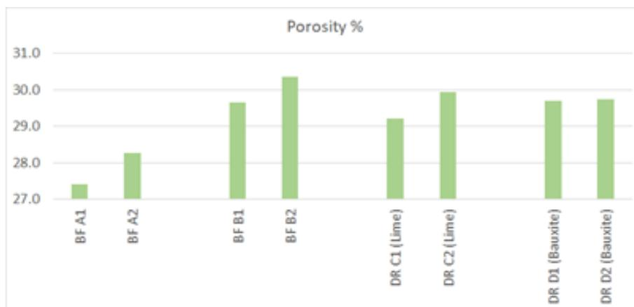
Figure 2. Porosity measurement of BF and DR grade pellets.
