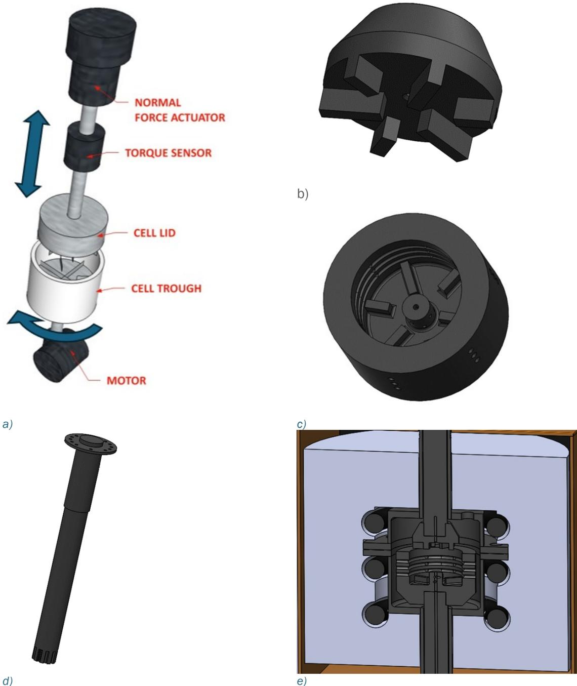
Figure 18. Details of the designed set-up: a) functional scheme; b) lid; c) trough; d) upper rod; e) measuring chamber in the oven.
