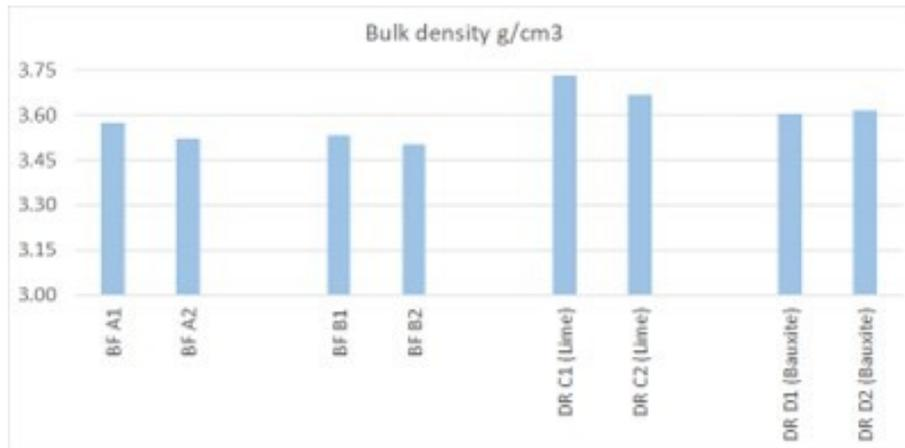
Figure 2. Bulk density measurement of BF and DR grade pellets.
