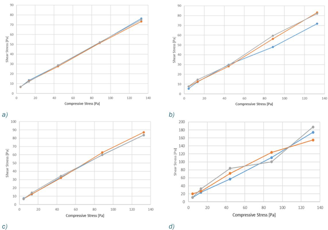
Figure 16. Yield loci at 5.0 kg pre-shear load: a) 6 mm wooden spheres, standard lid; b) 10 mm wooden spheres, standard lid; c) 10 mm wooden spheres, modified lid; d) Iron ore pellets, modified lid.
