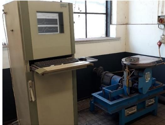
Figure 9. Determination of the cold crushing strength.
