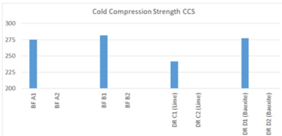
Figure 10. Cold Compression Strength of BF and DR grade pellets.
