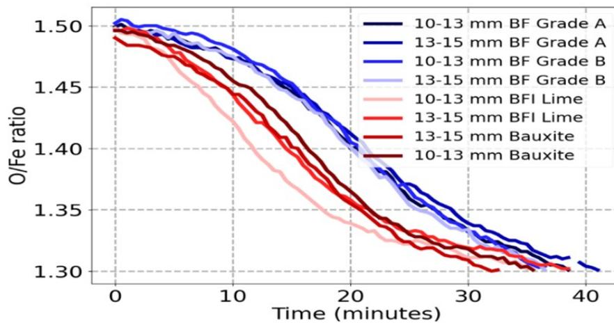
Figure 14. Reduction speed of BF and DR grade pellets under BF conditions.
