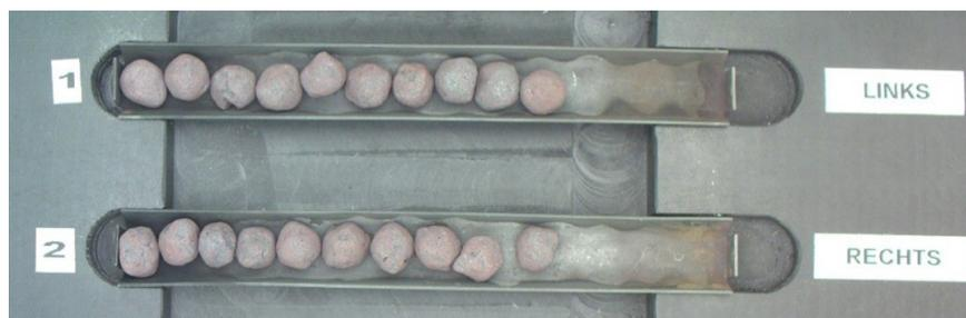
Figure 13. Swelling observation on BF grade pellet B1 (10-13 mm).
