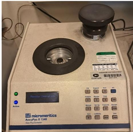
Figure 4. AccuPyc II 1340 device for measuring density.
