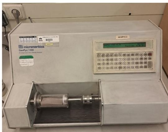
Figure 1. GeoPyc 1360 device for pellets porosity measurement.
