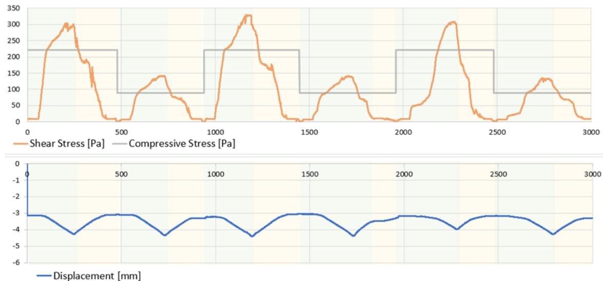
Figure 17. Raw data time series obtained with the Schulze Ring shear tester loaded with iron ore pellets, using the modified lid, using a pre-shearing load of 5 kg and a reduced pre-shear duration of 100 s. Regions characterized by normal trough rotation are green; those characterized by counter rotation are yellow.
