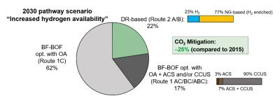
Since the availability of alternative carbon sources in 2030 is not yet clear, it was also assumed that fewer alternative carbon sources would be utilised. The specific CO<sub>2</sub> mitigation in the BF-BOFroute optimised by "other
